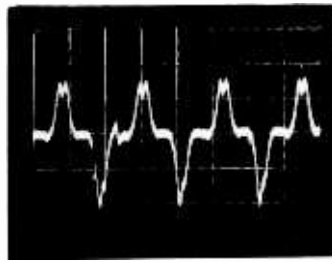
B. Excessive CT RECORD current.
